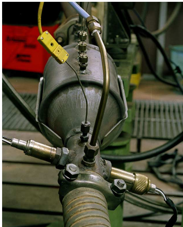
Fig. 2. Three-way catalytic converter equipped with a lambda probe (on the left) and a gas sensor (on the right).
